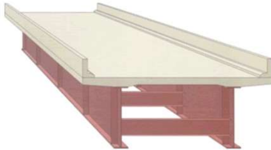
CIP Concrete Slab
