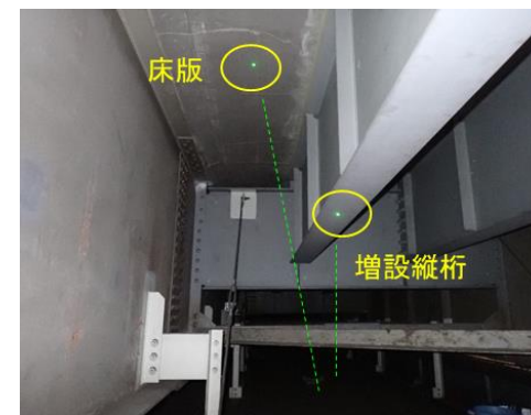
Measurement of deflection by laser Doppler
