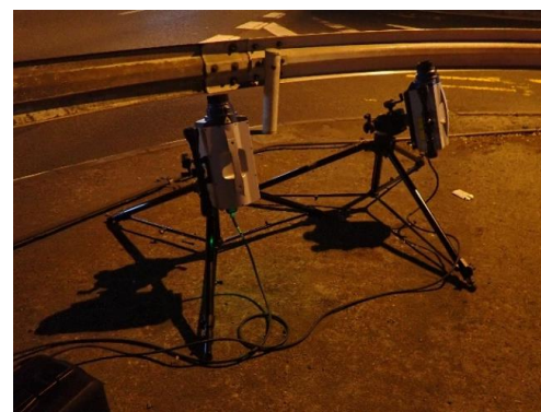
Measurement of deflection by laser Doppler
